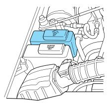
Only use a washer fluid that meets Ford specifications. Refer to *Lubricant specifications* in the *Capacities and specifications* chapter.
